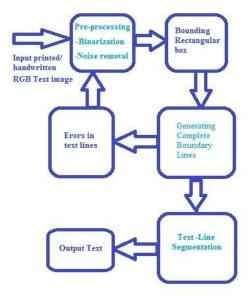
Fig. 2 Flowchart for line segmentation process
